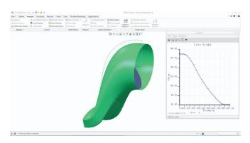
The trial-and-error approach to find the desired cross-sectional area along a curve can be extremely time-consuming, but with Creo BMX, it's fast and easy.
